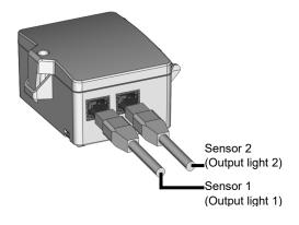
Two RJ45 sockets are integrated in the enclosure, this allows 2 light sensors to be connected with a shielded RJ45 cable of up to 10 m in length.
