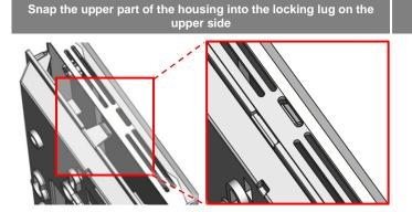
Fix the upper part of the housing on the underside with the
