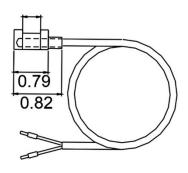
Connection housing USE-S optional (Type PR25+ passive)
